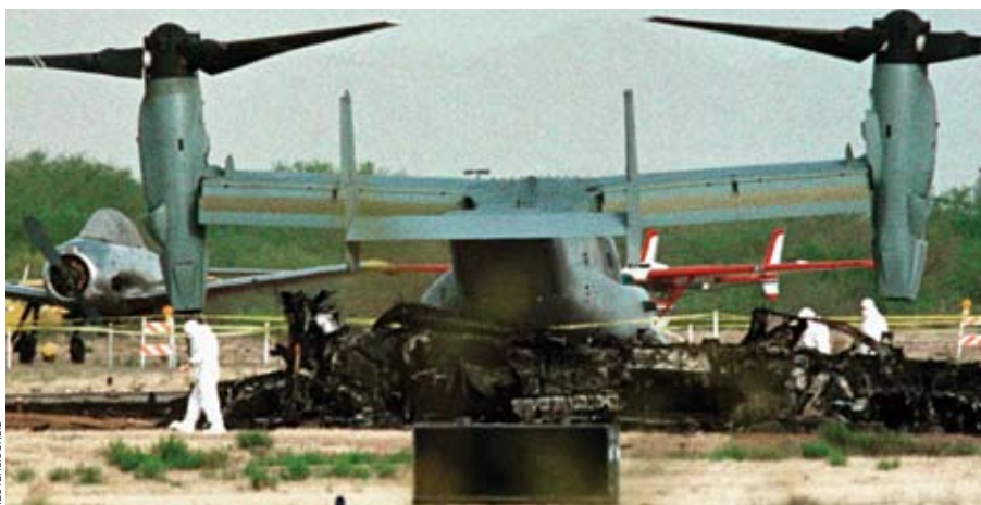
Dating to 1981, the joint Army/Marine Corps JVX program evolved into the MV-22 tiltrotor Osprey, a program nearly terminated 20 years later. Because of shortcuts to save time, only one-third of critical tests had been performed, resulting at least in part in an April 2000 crash that killed 19 Marines. Another crash that December brought the program to a halt, but it recovered and is expected to join Marine medium-lift forces shortly.
